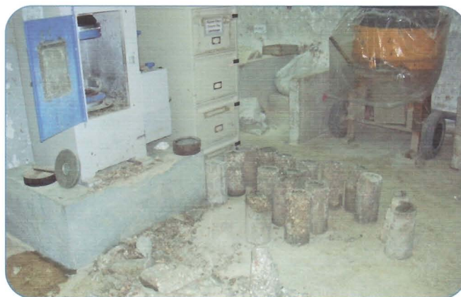
• Concrete cylinders for mechanical tests (crushing) at ACTS
